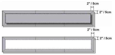
4. Cut along lines to make relief cuts, then carefully lift and pull center length cuts first using a chisel, then work into corners to remove end pieces last.
